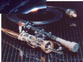
Arcjets on Telstar IV (Lockheed - US Commercial)
