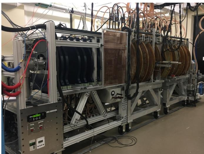
The PHase Space Mapping (PHASMA) experiment at WVU; measures distribution functions of both ions and electrons in a space-relevant plasma (e.g., Shi et al., Phys. Rev. Lett., 128, 025002, 2022)
